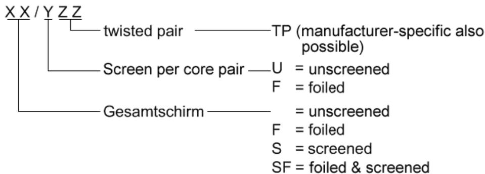
Figure 4-1: Cable structure according to ISO/IEC11801
