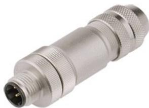
Figure 4-7: Connector EN61076-2-101, type D, four-pin, screened
