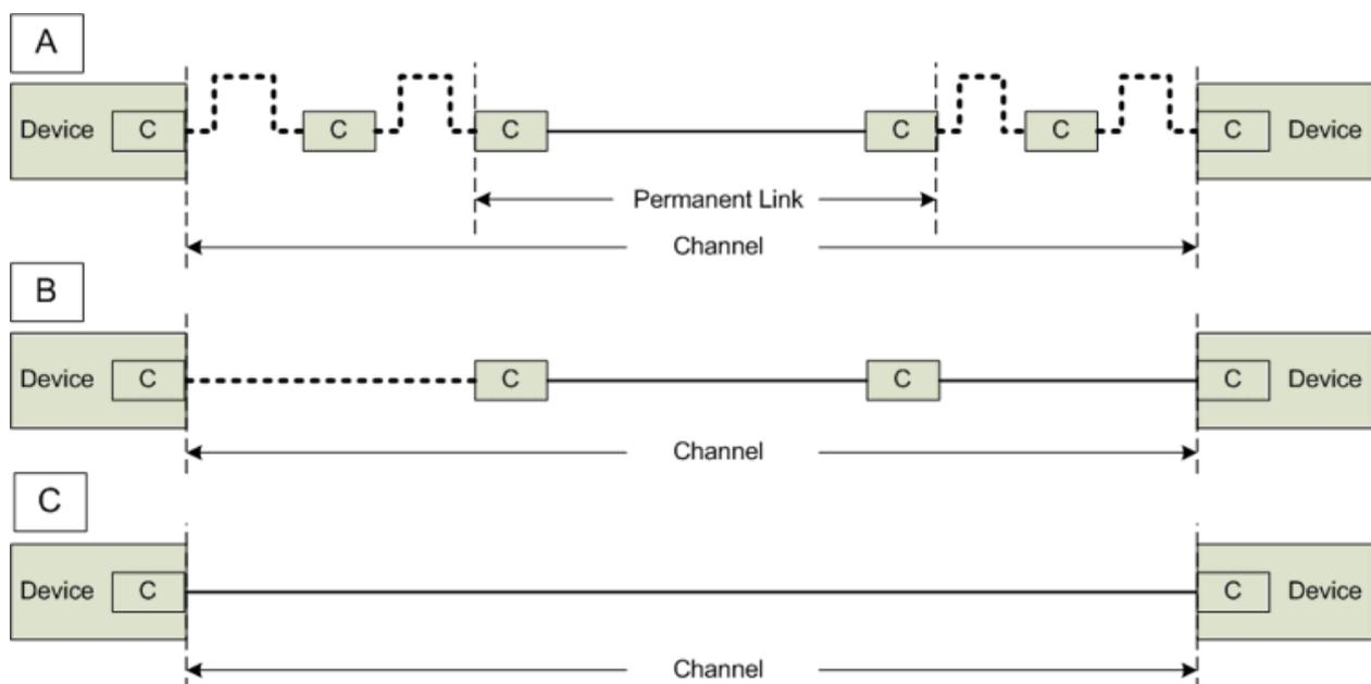
Figure 3-2: Models for the sections of a transmission link (channel):
